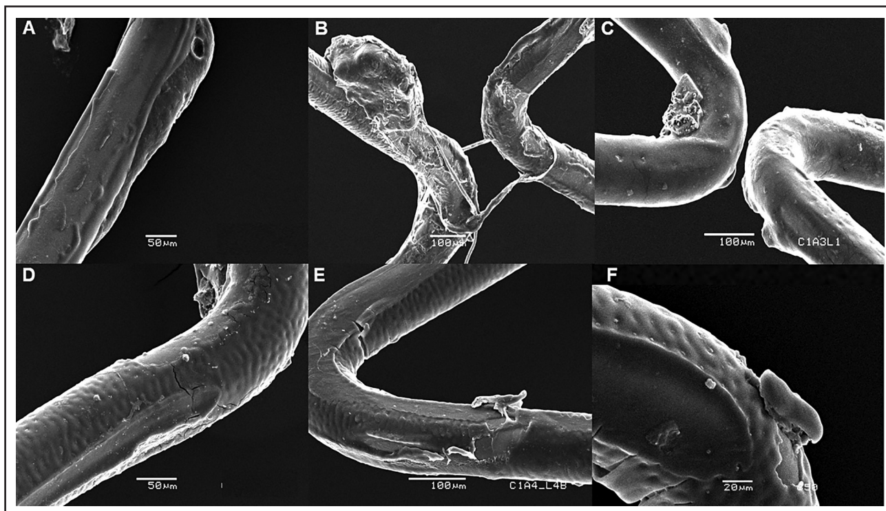
Figure 1. Examples of Onyx Frontier drug-eluting stent polymer coating irregularities observed by scanning electron microscopy.
