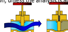
Gate Valve Opened
