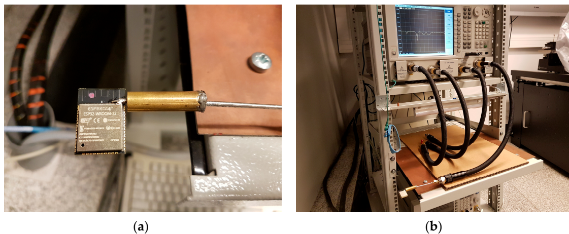
Figure 5. The laboratory measurements of the S11 parameter: (a) the sleeve balun choke used to suppress unwanted surface currents propagating onto the outer shield of the feeding cable and (b) equipment used during the S11 measurements.
