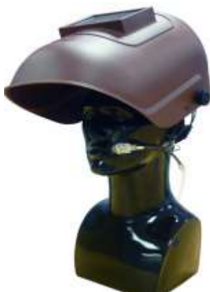
Figure 8. Mini-sampler and headset on worker (© Copyright 2018 SKC Inc.)
