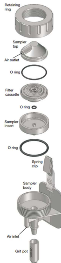
Figure 3. Configuration for plastic cyclone sampler and cassette
