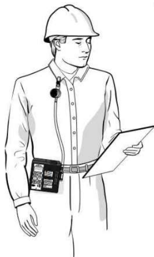
Figure 6. IOM sampler and pump on worker (other than welders) (© Copyright 2018 SKC Inc.)
