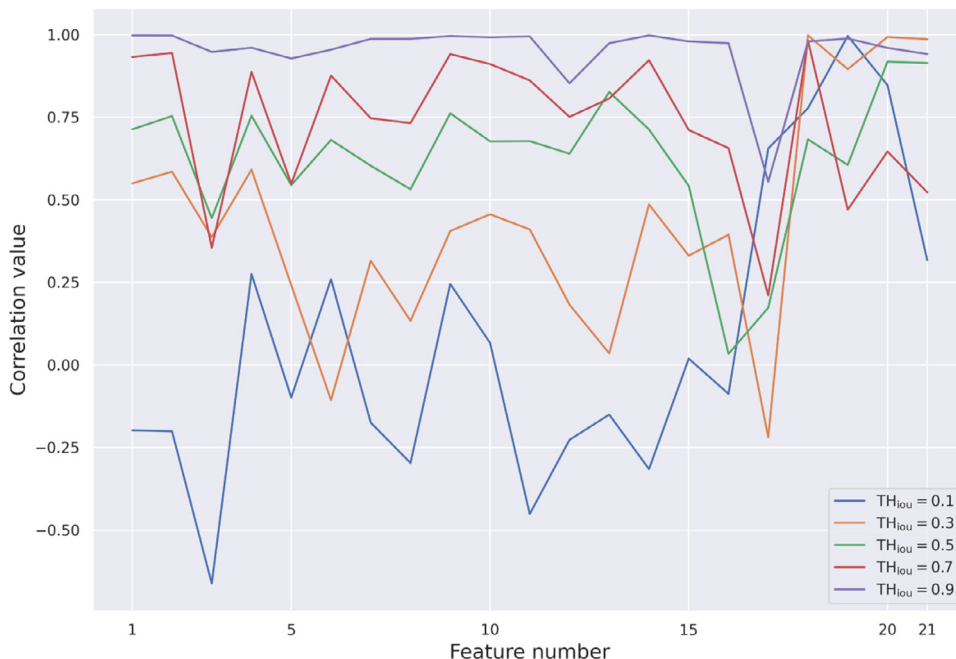
Fig. 8. Correlation between instantaneous features derived from ground-truth segmentation masks and those derived from 3D CNN segmentations, as a function of IoU. As can be observed, for most of the features, correlation is strong (higher than 0.5) when TH_{iou} \geq 0.5 . It should be also noticed, however, that those features related to the cell orientation with respect to that of the bloodstream (15–17) exhibit a higher sensitivity to TH_{iou} .
