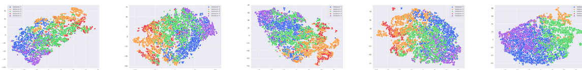
Fig. 24. Sensitivity of the explainability to the precision operation point: qualitative analysis. t-SNE diagrams for several precision operation points. From left to right: 95%, 92.5%, 90%, 87.5% and 85%. It should be noted that for 90% of precision the t-SNE topology begins to change and for 85% the 4th behavior disappears.
