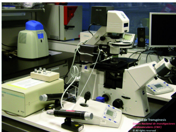
Zeiss AxioObserver-D1 optical inverted microscope and motorized micromanipulators used for the production of genetically-modified mice.
